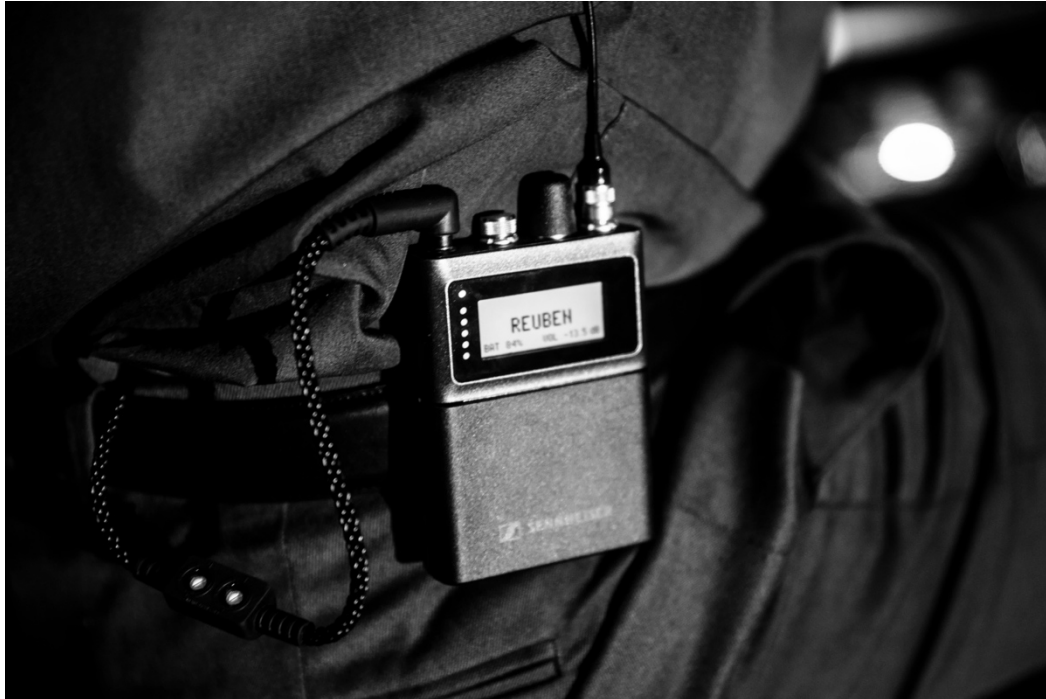
The Spectera bodypack combines microphone transmission and in-ear monitoring in a single bidirectional device, reducing set-up time and streamlining operations.
